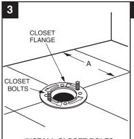
INSTALL CLOSET BOLTS Install closet bolts in flange channel, turn 90°, and slide into place 6" (152mm) apart and parallel to wall.
