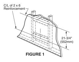
Using a level and square measure, mark the mounting hole locations. With assistance, hold the mirror and drill two 1/8" (3 mm) holes into the wall and install screws as described above. See Figure 1.
