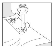
Use a screwdriver to tighten bolt.
