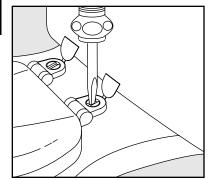
Use a screwdriver to tighten bolt.
