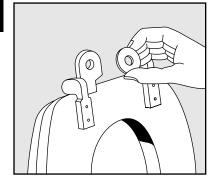
Attach washer to bottom of hinge.
