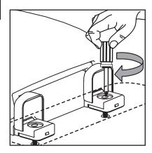
Tighten the bolts using a screwdriver. DO NOT OVERTIGHTEN.
