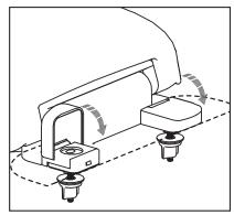
Close the hinge covers. The seat will not work if the hinge covers are not closed tightly.
