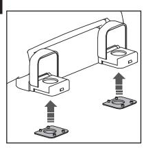
Install rubber base to seat post hinges.
