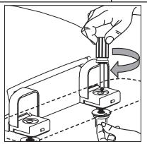
Thread the nuts onto the bolts. Tighten the bolts using a screwdriver. DO NOT OVERTIGHTEN.
