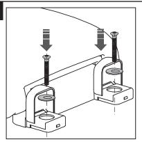
Slip the bolts through the washers, then through the hinge holes.
