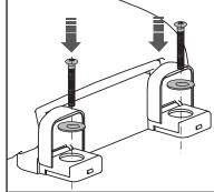
Slip the bolts through the washers, then through the hinge holes.
