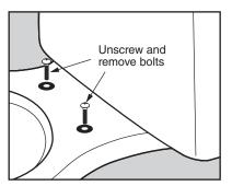
Once grommet is in place, unscrew and remove bolts and keep nearby for step 5.
