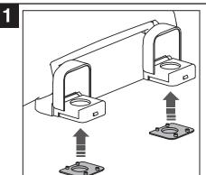
Install rubber base to seat post hinges.
