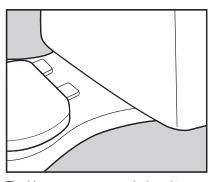
The hinge cap covers are designed to snap lock on to the hinge. Position the hinge covers and push down on the cover.
