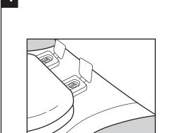
With the plastic bolts installed, thread the winged plastic nuts on to the bolts.
