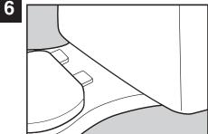
The hinge cap covers are designed to snap lock on to the hinge. Position the hinge covers and push down on the cover.
