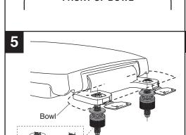
When closed nuts lock onto threads allowing final tightening with screwdriver or supplied attachment handles.
