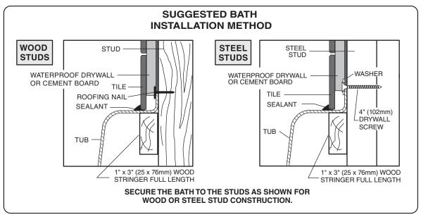
**C.)** Any finish material such as tile or wallboard must be self-supporting if it contacts the deck of the bath. Flooring will be butted against the bottom of the tub apron, also holding the tub in place.
