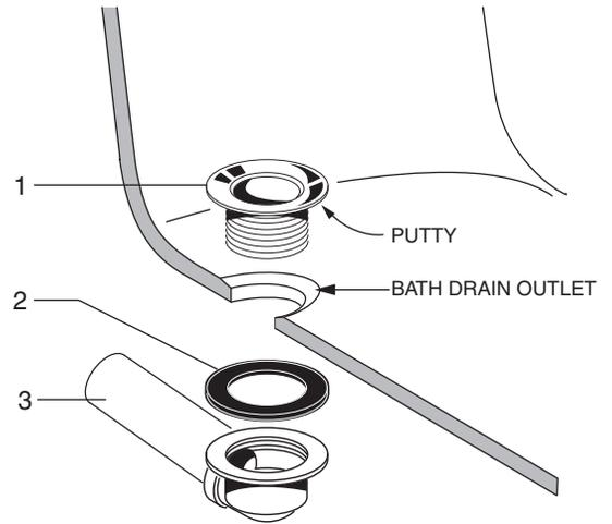
**NOTE:** TUB IS SHOWN CUT AWAY FOR CLARITY OF INSTALLATION.
