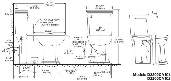
**IMPORTANT:** Water supply on the wall is required at 3" (76 or 229 mm) from centerline of the toilet (see rough-in). First suggested position is hidden behind the toilet. The geometry of the toilet gives space for this installation. The second suggested position is next to the toilet. Between these two positions, the space for the supply between wall and toilet is limited to 3-1/2" (89 mm). In this case, check your supply and hose dimensions.
