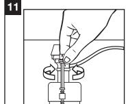
Turn on water supply. Submerge the FLOAT CUP under the water for 30 seconds. Adjust the water to desired level by turning WATER LEVEL ADJUSTMENT ROD and moving FLOAT CUP up or down.
