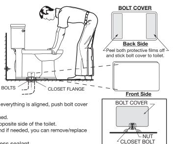
For Tanks/Bowls using Speed Connect System (Tank mounting bolts pre-installed).
