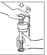
Replace TOP by engaging lugs and rotating 1/8 turn clockwise. MAKE CERTAIN TIP IS TURNED TO THE LOCKED POSITION. VALVE MAY NOT TURN ON IF TOP IS NOT FULLY TURNED TO THE LOCKED POS
