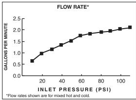
1.8 gpm/6.8 L/min. FLOW RATE
