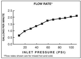
1.8 gpm/6.8 L/min. FLOW RATE
