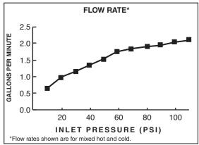
1.8 gpm/6.8 L/min. FLOW RATE
