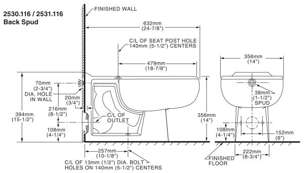
WASTE OUTLET SEAL RING MUST BE NEOPRENE OR GRAPHITE-FELT (WAX RING NOT RECOMMENDED).
