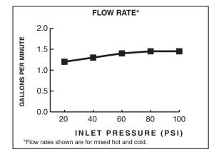
1.5 gpm/5.7 L/min. FLOW RATE
