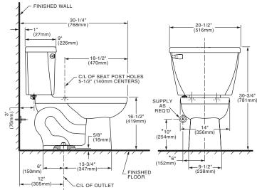
THIS TOILET IS DESIGNED TO ROUGH-IN AT A MINIMUM DIMENSION OF 305mm (12") FROM FINISHED WALL TO C/L OF OUTLET. SUPPLY NOT INCLUDED WITH FIXTURE AND MUST BE ORDERED
