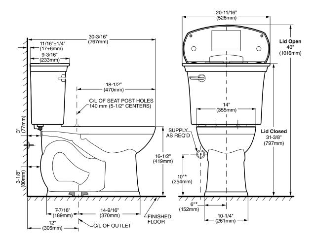
NOTES: THIS TOILET IS DESIGNED TO ROUGH-IN AT A MINIMUM DIMENSION OF 305mm (12") FROM FINISHED WALL TO C/L OF OUTLET. SUPPLY NOT INCLUDED WITH FIXTURE AND MUST BE ORDERED SEPARATELY. \* DIMENSION SHOWN FOR LOCATION OF SUPPLY IS SUGGESTED.
