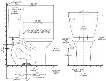
THIS COMBINATION IS DESIGNED TO ROUGH-IN AT A MINIMUM DIMENSION OF 305MM (12") FROM FINISHED WALL TO C/L OF OUTLET.
