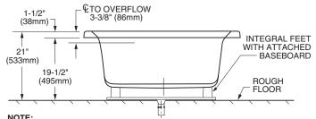
NOTE: THE MUST PROVIDE 12" X 24" ACCESS OPENING FOR SERVICING AIR BLOWER, PUMP MOTOR, WHIRLPOOL HEATER, AND LIGHTING SYSTEM.
