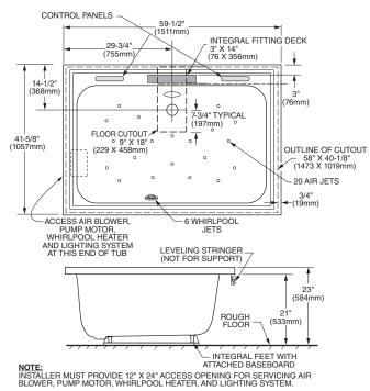
THIS MODEL INCLUDES A DRAIN ASSEMBLY. OTHER DRAIN ASSEMBLIES CANNOT BE USED. REVIEW DRAIN INSTALLATION DETAILS IN THE DOCUMENT TO FULLY UNDERSTAND FLOOR CUTOUT REQUIREMENTS.
