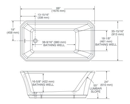
Freestanding tubs use wall-mounted or freestanding faucets. The waste and overflow assembly is concealed between the walls of the tub, eliminating the need for a decorative exposed drain kit.
