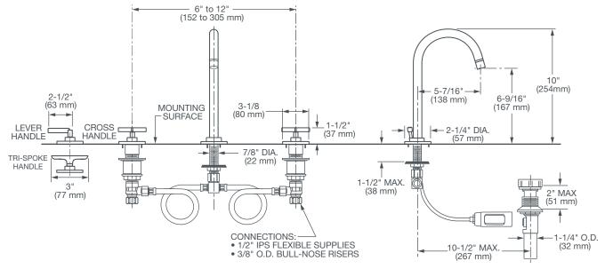
NOTE: MOUNTING HOLES ARE 1-3/8" DIA. (35 mm)
