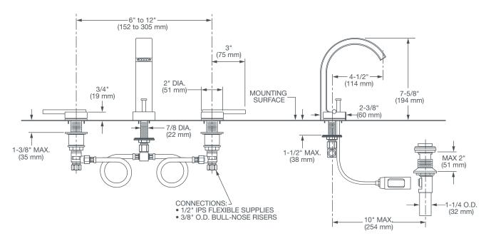
NOTE: MOUNTING HOLES ARE 1-3/8" DIA. (35 mm)
