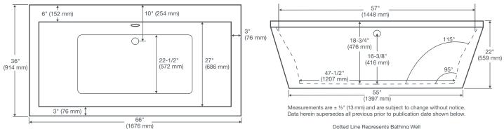
Freestanding tubs use wall-mounted or freestanding faucets. The waste and overflow assembly is concealed between the walls of the tub, eliminating the need for a decorative exposed drain kit.
