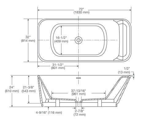
Freestanding tubs use wall-mounted or freestanding faucets. The waste and overflow assembly is concealed between the walls of the tub, eliminating the need for a decorative exposed drain kit.
