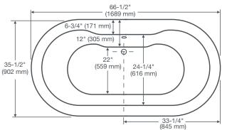
Freestanding tubs use wall-mounted or freestanding faucets. The waste and overflow assembly is concealed between the walls of the tub, eliminating the need for a decorative exposed drain kit. Dotted Line Represents Bathing Well
