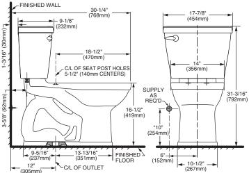
NOTES: THIS TOILET IS DESIGNED TO ROUGH-IN AT A MINIMUM DIMENSION OF 305MM (12") FROM FINISHED WALL TO C/L OF OUTLET. SUPPLY NOT INCLUDED WITH FIXTURE AND MUST BE ORDERED SEPARATELY
