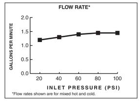
1.5 gpm/5.7 L/min. FLOW RATE
