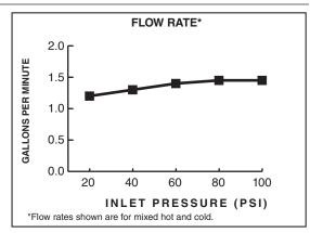
1.5 gpm/5.7 L/min. FLOW RATE
