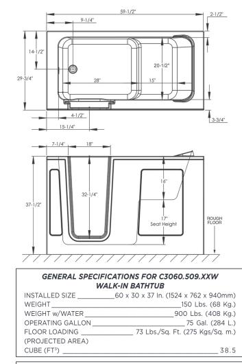
**To Be Specified - Required:** Drain Configuration: Left (L) or Right (R)
