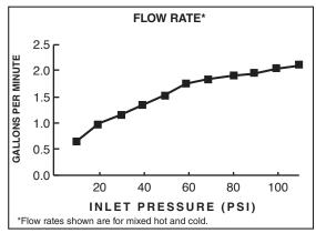
1.8 gpm/6.8 L/min. FLOW RATE
