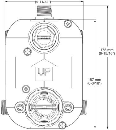
**Exclusive Plaster Guard:** Plaster guard is designed to protect valve and act as a guide during installation.
