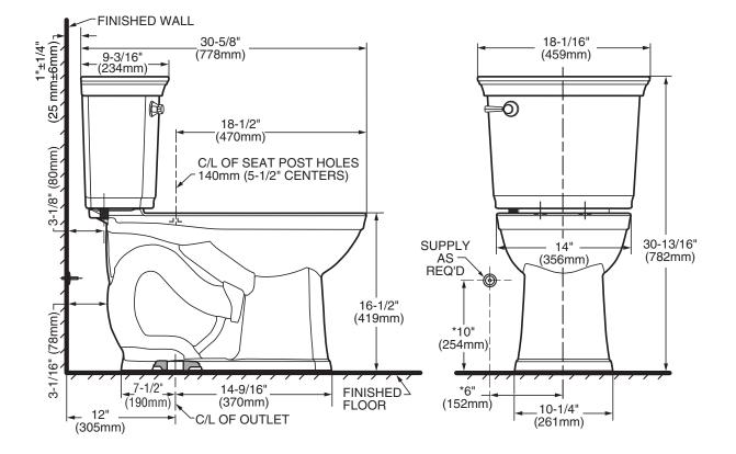
NOTES: THIS TOILET IS DESIGNED TO ROUGH-IN AT A MINIMUM DIMENSION OF 305mm (12") FROM FINISHED WALL TO C/L OF OUTLET. SUPPLY NOT INCLUDED WITH FIXTURE AND MUST BE ORDERED SEPARATELY. \* DIMENSION SHOWN FOR LOCATION OF SUPPLY IS SUGGESTED.
