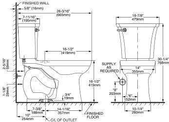
THIS COMBINATION IS DESIGNED TO ROUGH-IN AT A MINIMUM DIMENSION OF 254MM (10") FROM FINISHED WALL TO C/L OF OUTLET.
