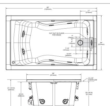
DIMENSIONS OF FIXTURES ARE NOMINAL AND MAY VARY WITHIN THE RANGE OF TOLERANCES ESTABLISHED BY ANSI STANDARDS 7124 1 AND A112 19 7.
