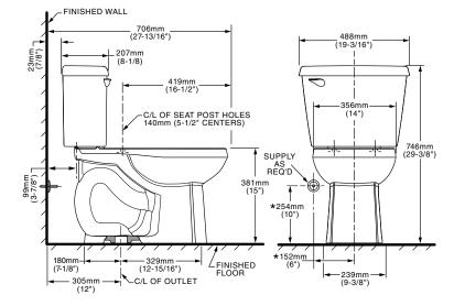
THIS TOILET IS DESIGNED TO ROUGH-IN AT A MINIMUM DIMENSION OF 305MM (12") FROM FINISHED WALL TO C/L OF OUTLET. SUPPLY NOT INCLUDED WITH FIXTURE AND MUST BE ORDERED SEPARATELY. \* DIMENSION SHOWN FOR LOCATION OF SUPPLY IS SUGGESTED.
