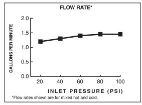
1.5 gpm/5.7 L/min. FLOW RATE
