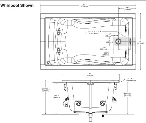
DIMENSIONS OF FIXTURES ARE NOMINAL AND MAY VARY WITHIN THE RANGE OF TOLERANCES ESTABLISHED BY ANSI STANDARDS Z124.1 AND A112.19.7.
