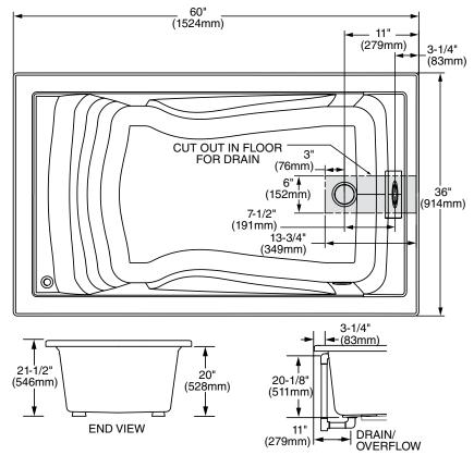
DIMENSIONS OF FIXTURES ARE NOMINAL AND MAY VARY WITHIN THE RANGE OF TOLERANCES ESTABLISHED BY ANSI STANDARDS Z124.1.2 AND A112.19.7
