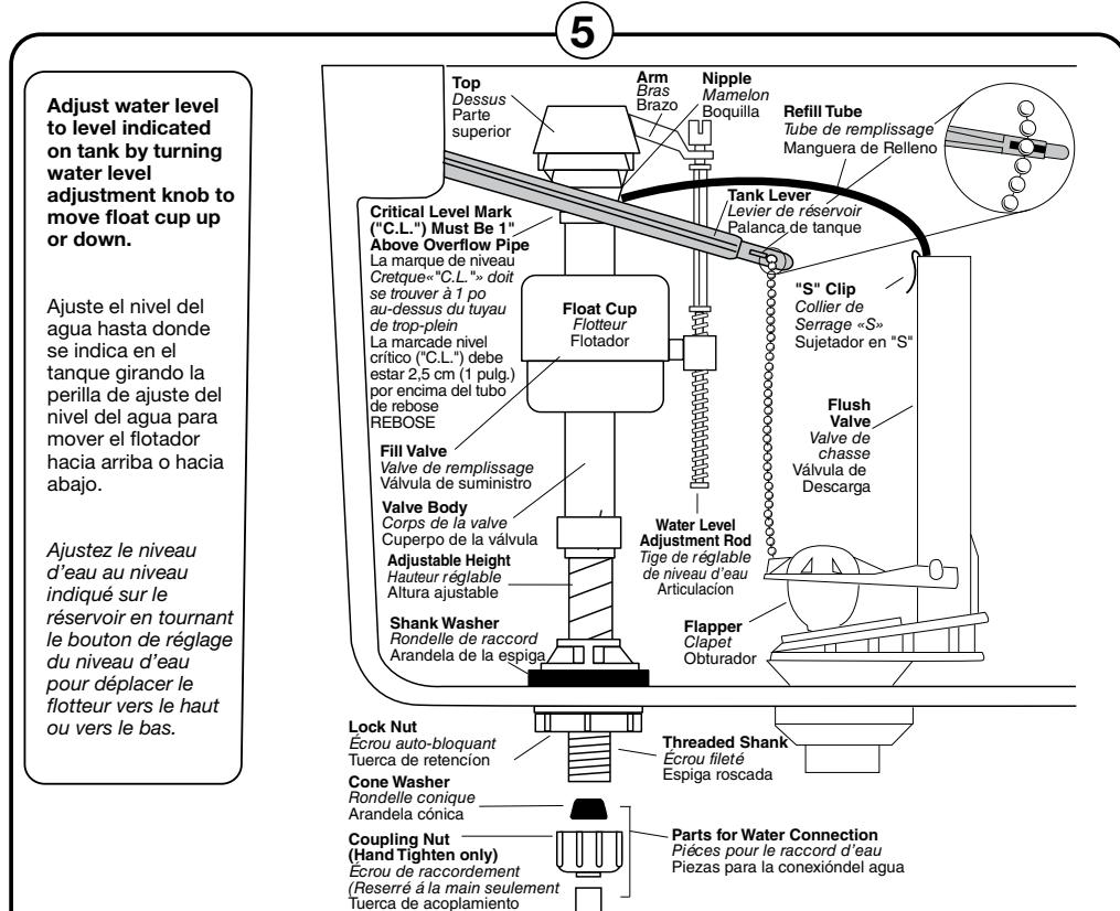
Adjust water level to level indicated on tank by turning water level adjustment knob to move float cup up or down.
