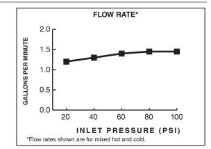
1.5 gpm/5.7 L/min. FLOW RATE
