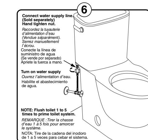
**WARNING:** Overtightening of water supply line nuts could result in breakage and potential flooding.
