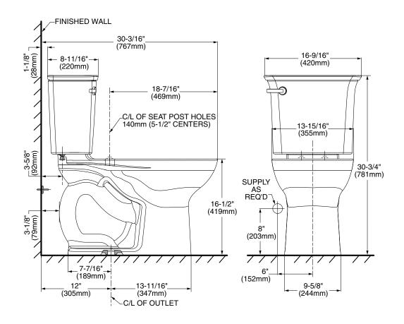
THIS TOILET IS DESIGNED TO ROUGH-IN AT A MINIMUM DIMENSION OF 305MM (12") FROM FINISHED WALL TO C/L OF OUTLET. SUPPLY NOT INCLUDED WITH FIXTURE AND MUST BE ORDERED SEPARATELY.
