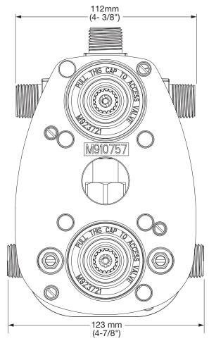
**Solid Brass Inlet Connections:** Fast and easy installation without adaptors reducing leak points - Easier and flameless installation (no soldering required)
