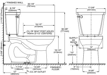
THIS COMBINATION IS DESIGNED TO ROUGH-IN AT A MINIMUM DIMENSION OF 305MM (12") FROM FINISHED WALL TO C/L OF OUTLET.
