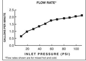
1.8 gpm/6.8 L/min. FLOW RATE
