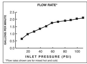
1.8 gpm/6.8 L/min. FLOW RATE
