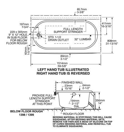
NOTE: Install this product according to the installation guide. ADA, CSA compliant when installed to the specific requirements of these regulations.
