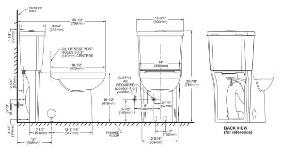
IMPORTANT: Water supply on the wall is required at 2-1/4" or 8" from centerline of the toilet (see rough-in). First suggested position is hidden behind the toilet. The geometry of the toilet gives space for this installation. The second suggested position is next to the toilet. Between these two positions, the space for the supply between wall and toilet is limited to 4-1/2". In this case, check your supply and hose dimensions.
