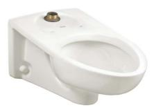
The wall-hung elongated flushometer bowl shall be made of vitreous china. Product shall be 26" in length, 14" in width, and 15" to 16-1/2" in height when installed on a wall-hung carrier by others. Product shall have a 12" x 10" water area. Product shall have 2-1/8" (54 mm) glazed trapway, and a 1-1/2" top or back spud. Product shall be available with or without bedpan lugs and with or without the EverClean surface.
